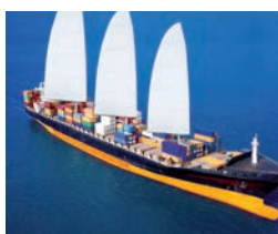
Rigid shipping sails Reducing fuel consumption with wind power
